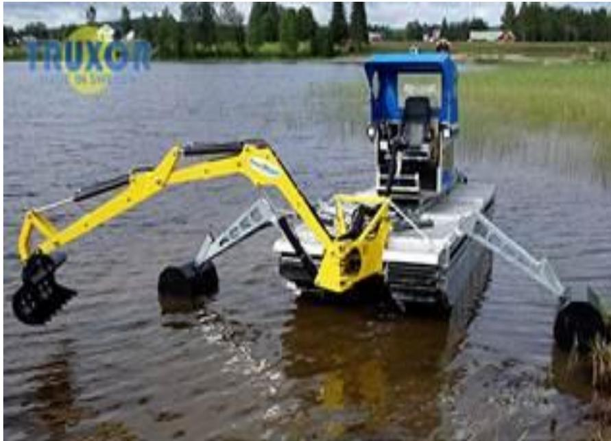
**The silt sampling machinery to be used to collect samples on the Parrett and Tone**
